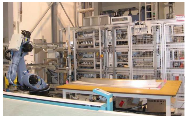
Process chain with continuous preforming machine, robot and compaction tool
